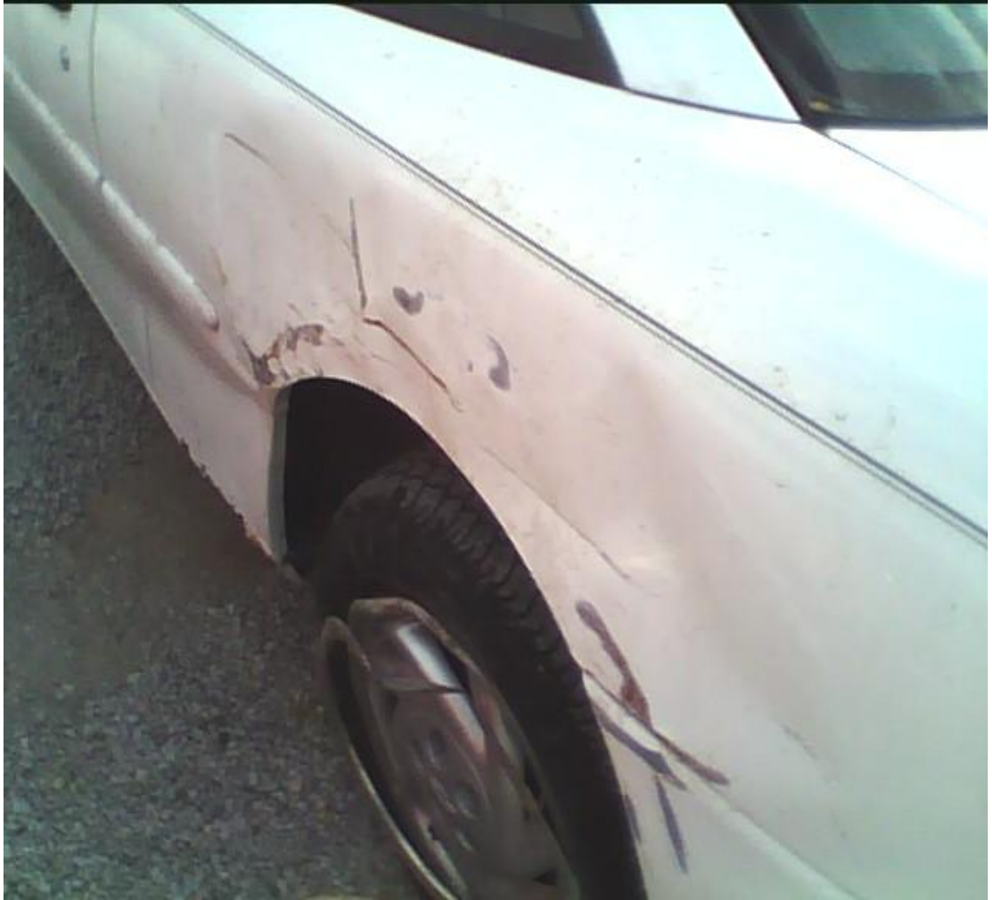
Note Defendants Vehicle that scraped concrete barrier and paint marks
