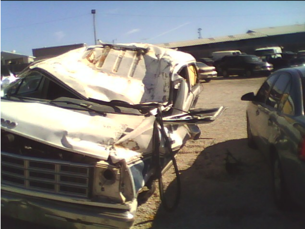
Figure 2 Roll over damage
